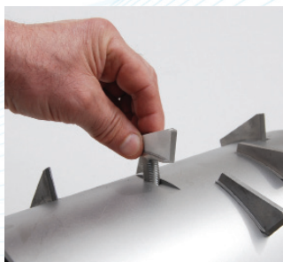
Individually replaceable teeth on drum.
